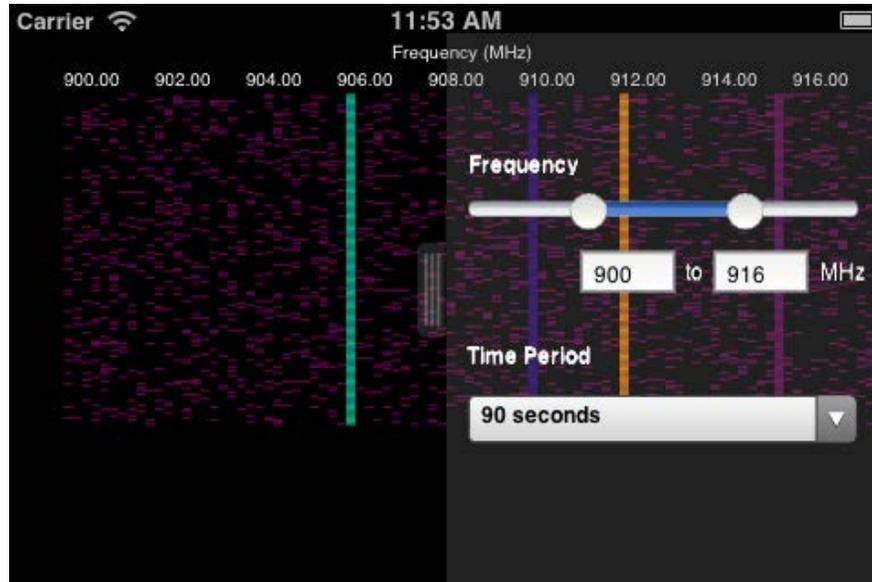
The frequency range selection is identical to that in the frequency plot mode. However, in this mode, the user must also select the time period for the historical data. The user is unlikely to care about the precise period (e.g., the difference between 37 and 38 seconds), but more the general scope of the display, so it was decided to present this option as a drop list with geometrically-increasing periods: 5 seconds, 10 seconds, 20 seconds, 30 seconds, 45 seconds, etc.
