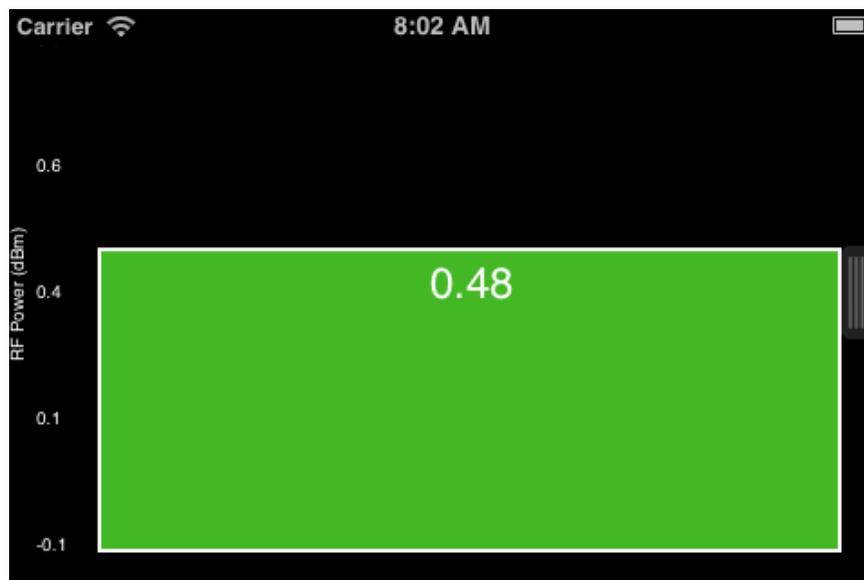
The color of the bar changes based on the reading – higher readings result in brighter, more “energetic” colors (in practice, this translates as brighter, more saturated, and closer to the red end of the spectrum). This allows the user to give most of their attention to something else – the controls of their transmitter, for example – while still tracking the power output from the corner of their eye.
