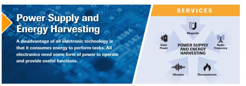
Many electronic products require portability or remote functionality far from AC line power. Since, in most cases, it is desirable to avoid using batteries that need changing on some regular interval, energy harvesting allows low power electronics to run indefinitely without external power. The device itself extracts power from the environment.
