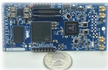
Figure 1: Vanteon vProtean Software Defined Radio (SDR)
