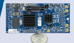
vProtean<sup>™</sup> is the flexible Wideband SDR for signal intelligence and multi-band processing applications. Its configurable, high performance, RF front end is frequency and bandwidth configurable, while its integrated RF transceiver provides optimal narrowband performance.
